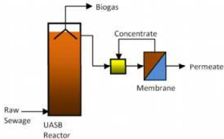
Figure 2. 6: UASB Post Effluent Polishing Using Membrane (ÖZGÜN, 2015).
