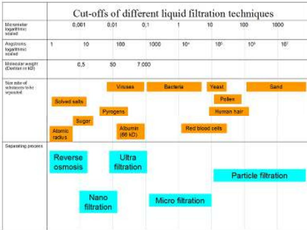
Figure 2. 5: Cut-offs of Different Liquid Filtration Technique (wikipedia.com).
