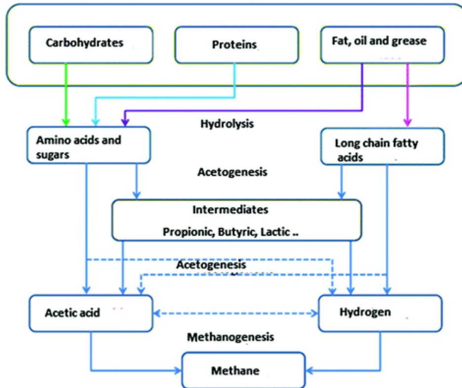
Figure 2. 1: Anaerobic Oxidation Process (Bajpai, 2017)
