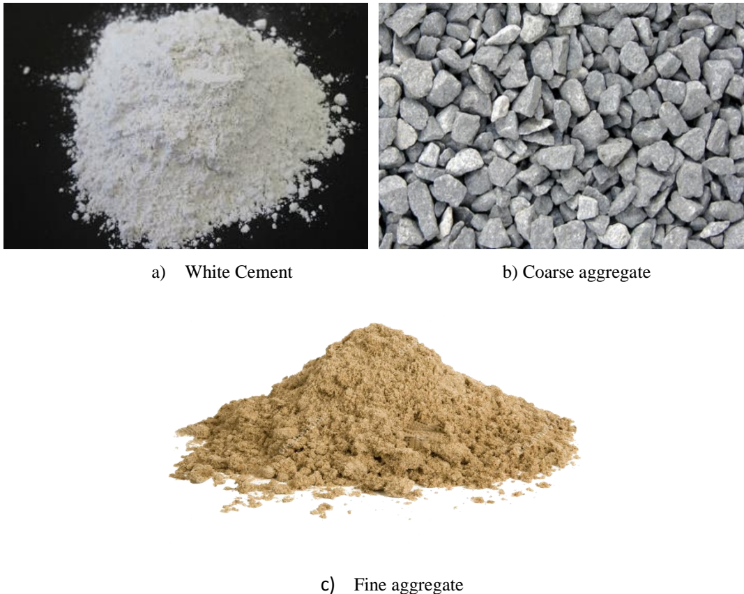
Figure 4. Constituents of cast stone mix
