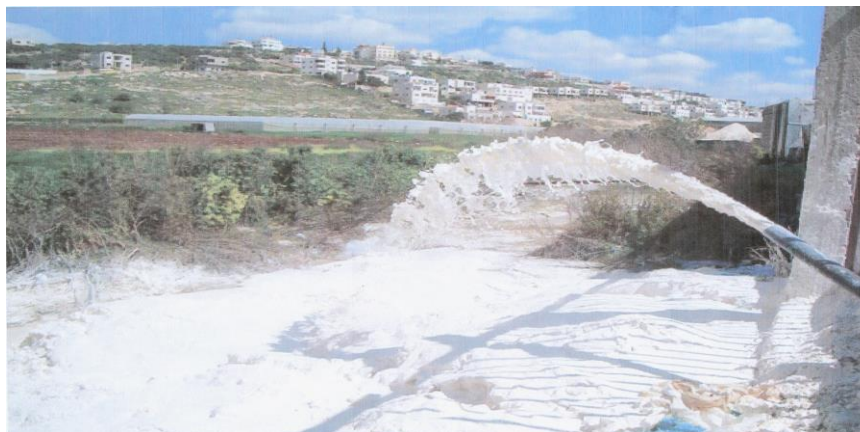
Figure 3. Discharge of stone slurry wastewater from stone cutting plant out in open areas
