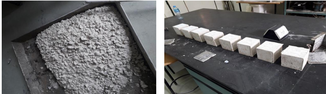
Figure 5. Fresh mix and hardened samples of cast stone mix
